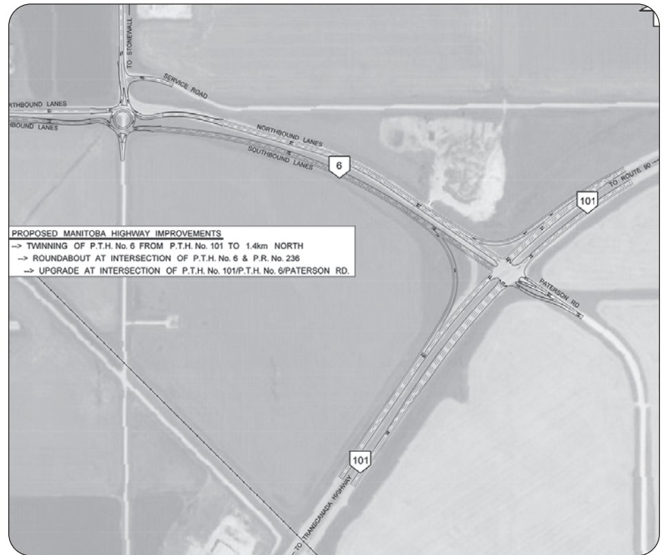
EXPRESS PHOTO SUBMITTED Proposed Manitoba Highway improvements include the twinning of PTH 6 from PTH 101, a roundabout at PTH 6 and PR 236 intersection and upgrade at intersection of PTH 101 and PTH 6 and Paterson Rd.
