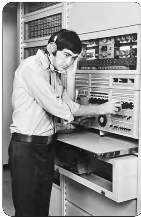
An employee of AEI Telecommunications with the racks that contain the switching equipment for the earlier versions of the control boards.
