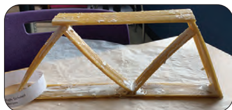
The physics class's winning bridge weighed under 350 grams yet supported 42.4 kilograms. Zachary Fedorchuk and Allan Dyker built it.
