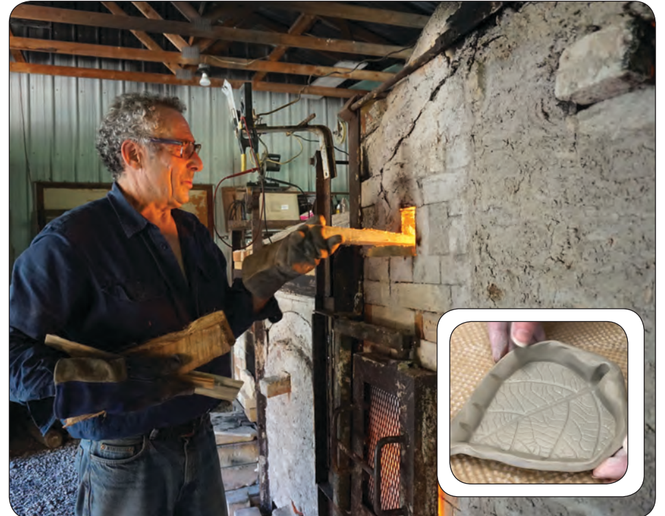
Alan Lacovetsky stokes the fire in his wood-burning kiln. Each firing takes approximately 30 hours, with wood needing to be fed to the stove every five to 10 minutes the entire time. Lacovetsky created the ceramic aspen leaf mould for Dawson.
