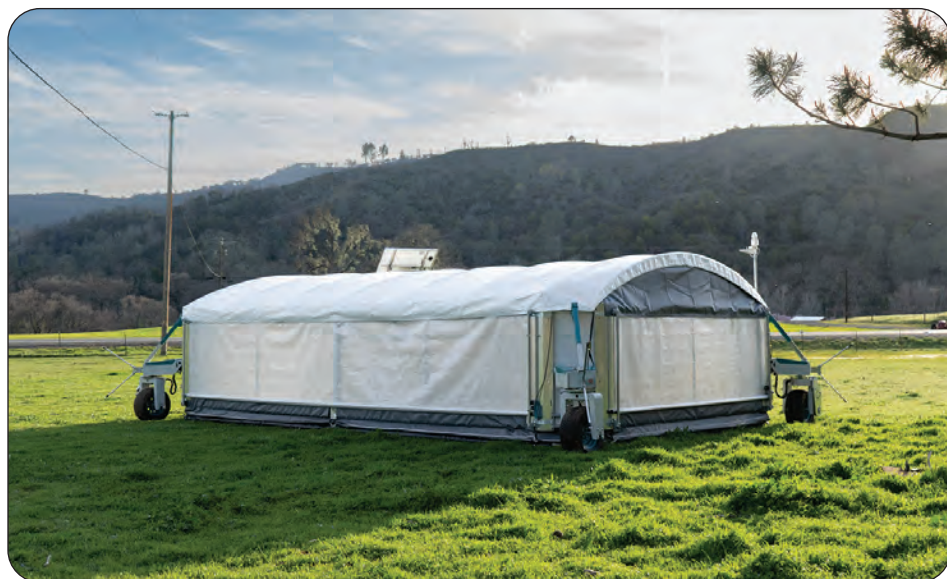
The ROVABARN autonomously moves birds to fresh pasture multiple times a day, handles automatic feeding and watering, provides automatic ventilation and is solar-powered, with connectivity to smartphones.
