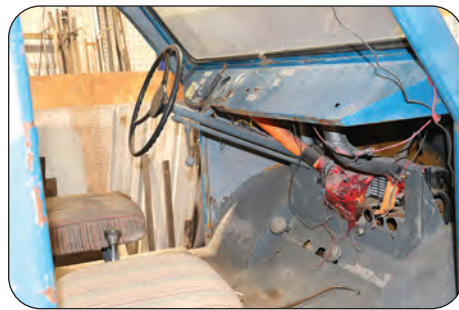
Bombardiers have a steering wheel and gas and brake pedals. Early models were standard with a clutch.
